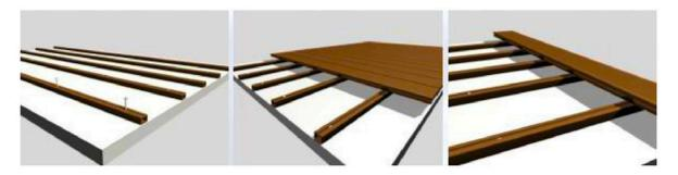
The WPC products' expansion rate is around 0.3% to 0.5% depends on different weather condition in different places, based on this expansion rate, there must be a gap always between two WPC products, as follows:
