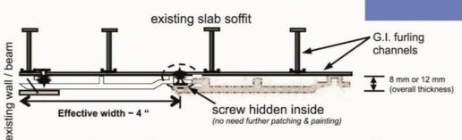
3-step Installation Method, Screw → Clip-in → Screw Again & repeat...
